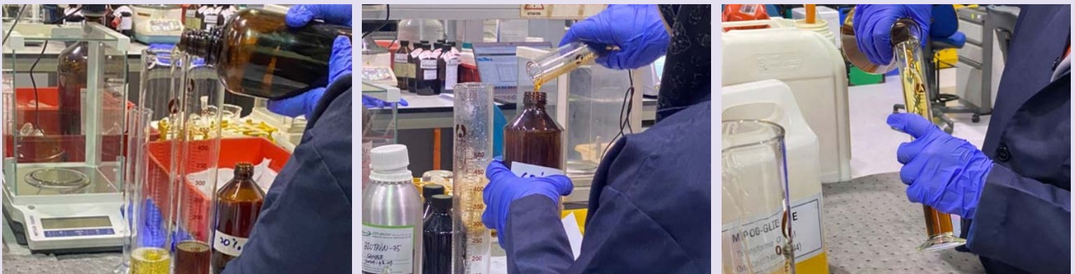
Research is underway to assess the feasibility of biodegradable, ester-based transformer oils, including palm oil-based variants, for use across different transformer applications and network conditions, with the aim of strengthening environmental risk management.
