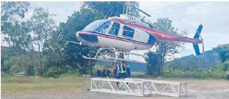
Helicopter being used to transport ERS components.
