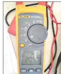
Voltage readings were taken before the change to a different phase was enacted.
