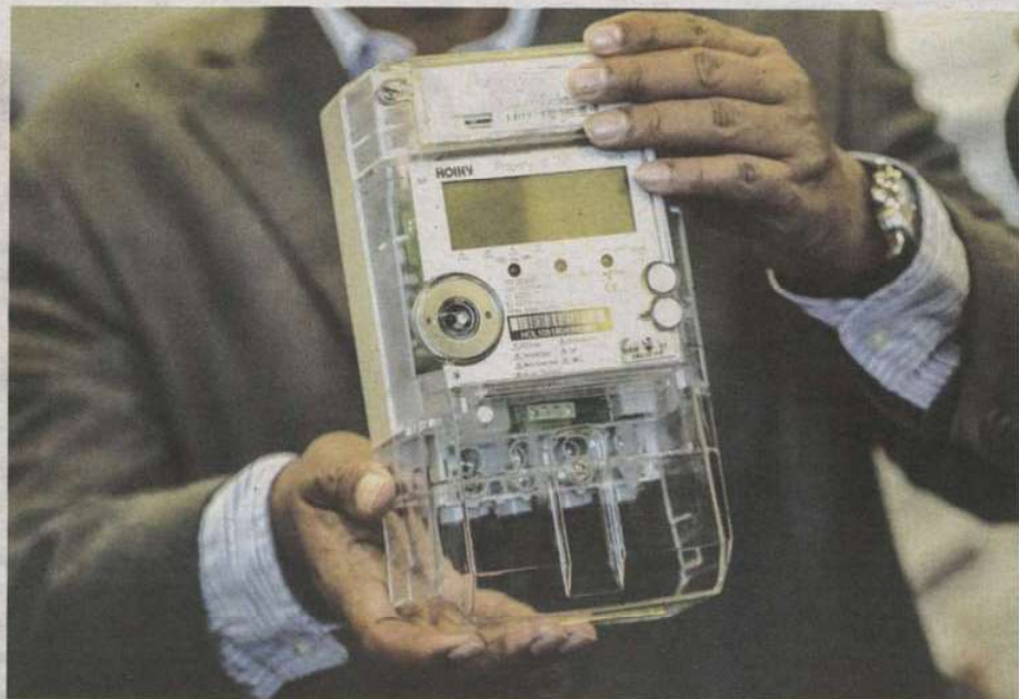
The AMI infrastructure architecture which uses smart meter allows for the device to communicate with the meter data management and head-end systems via the radio frequency mesh network
