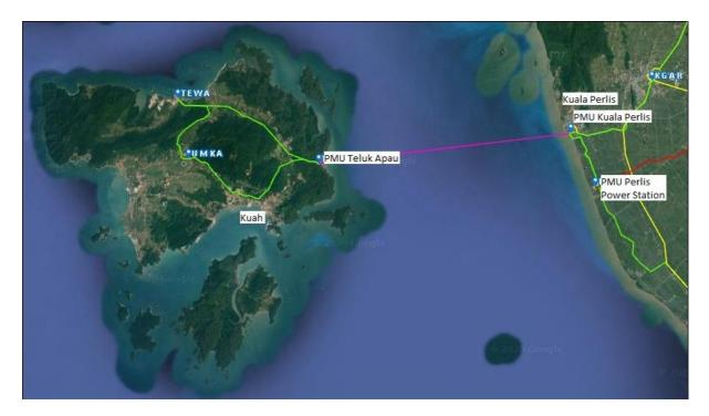
The 26.5km submarine cable is TNB's third high-voltage cable installed to connect the paradisiacal island with the National Grid.
